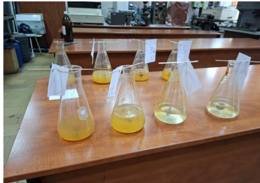
Fig. 5. Immersion of specimens into the test vessels.
