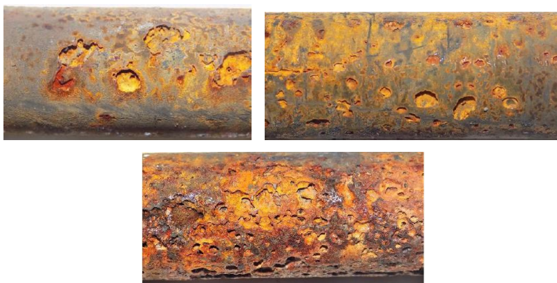
Fig. 9. Aspects of pitting corrosion and under-deposit corrosion (crevice and pitting cavities) – sample 1.
