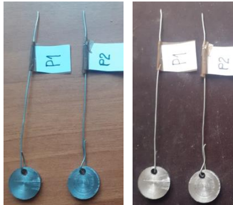
Fig. 4. Corrosion specimens prepared for insertion into the working fluid.
