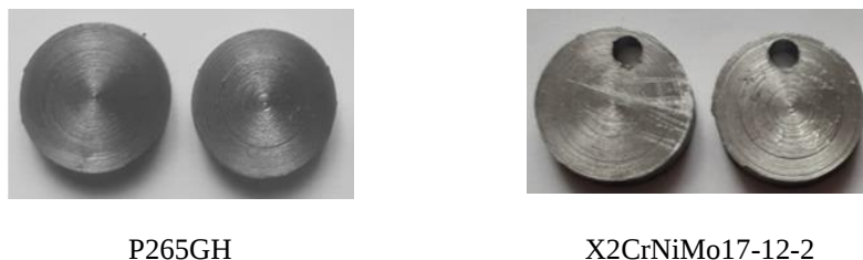
Fig. 2. Test specimens used for the corrosion evaluation.
