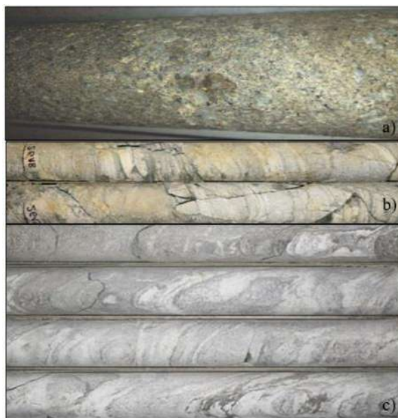
Figure 8 – Representative mechanical cores: a) Conglomerate; b) Breccia; c) Paleozoic
