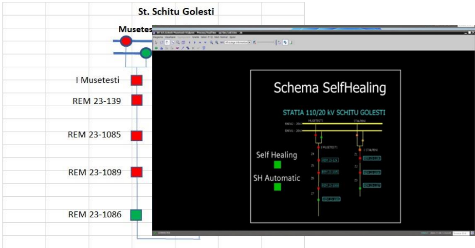
Fig. 3. Automation diagram for two MV lines (SCADA schematic capture).
