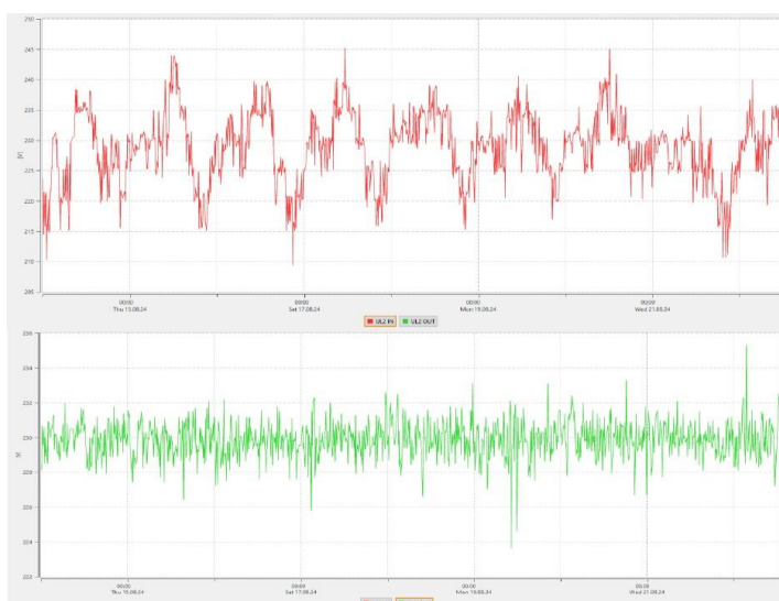
Figure 3. Voltage curves on phase 2 upstream (red) and downstream (green) of the regulator
