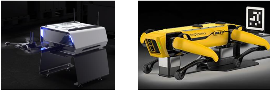
Figure 9. Self charging dock for autonomous systems [6]
