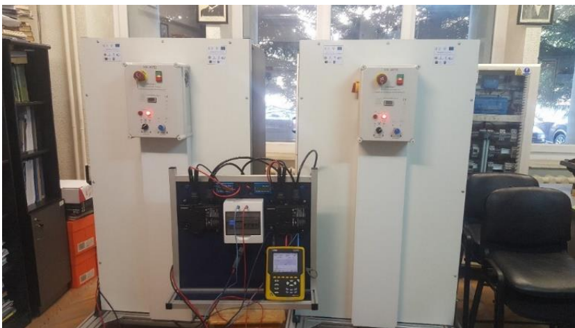
Figure 2. Experimental stand with two solar simulators
