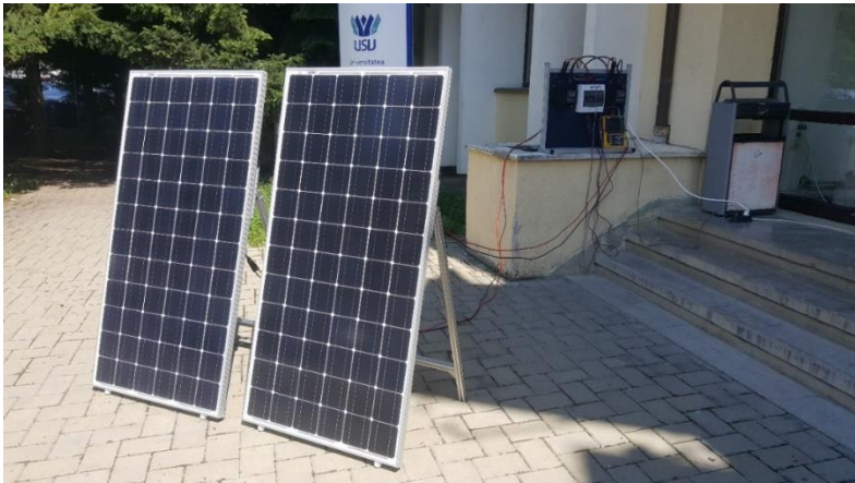
Figure 7. Photovoltaic panels and experimental stand in real climatic conditions.
