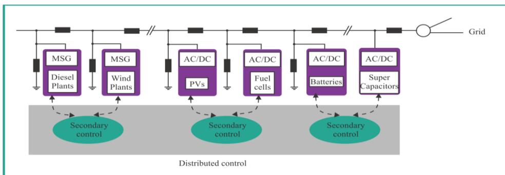
**Figure 1.** Structure of hybrid MG [9].
