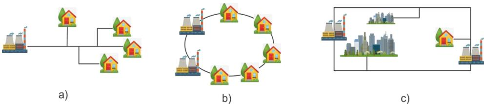
**Figure 2.** Electrical power distribution system [7]:
