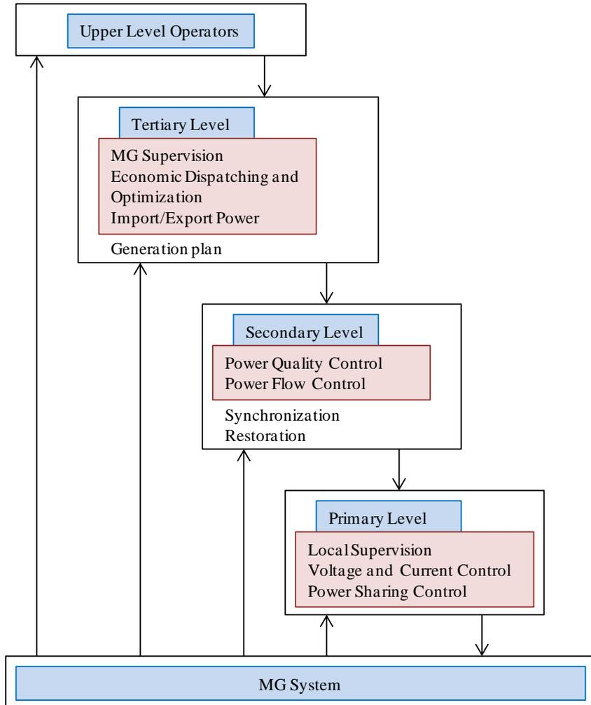
**Figure 6.** Control scheme - Schematic diagram.
