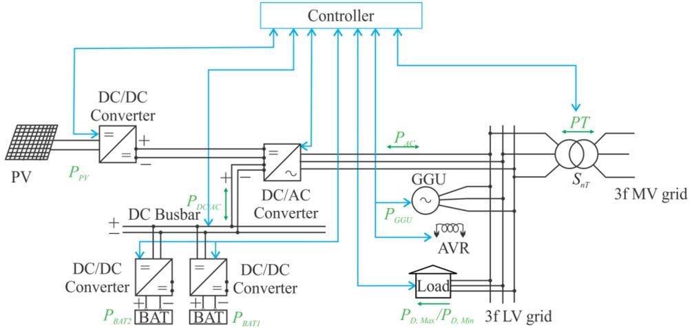
**Figure 5.** The real case MG structure.
