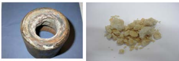
Figure 5 - Carbonate scale inside tubing ( foto left side ) and halit scale ( foto right side )
