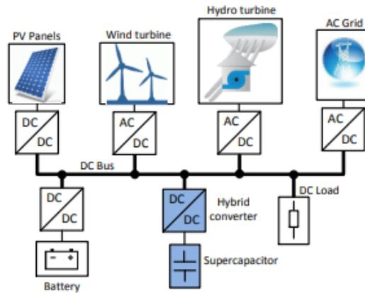
Figure 1 - Block structure of a microgrid network [2]
