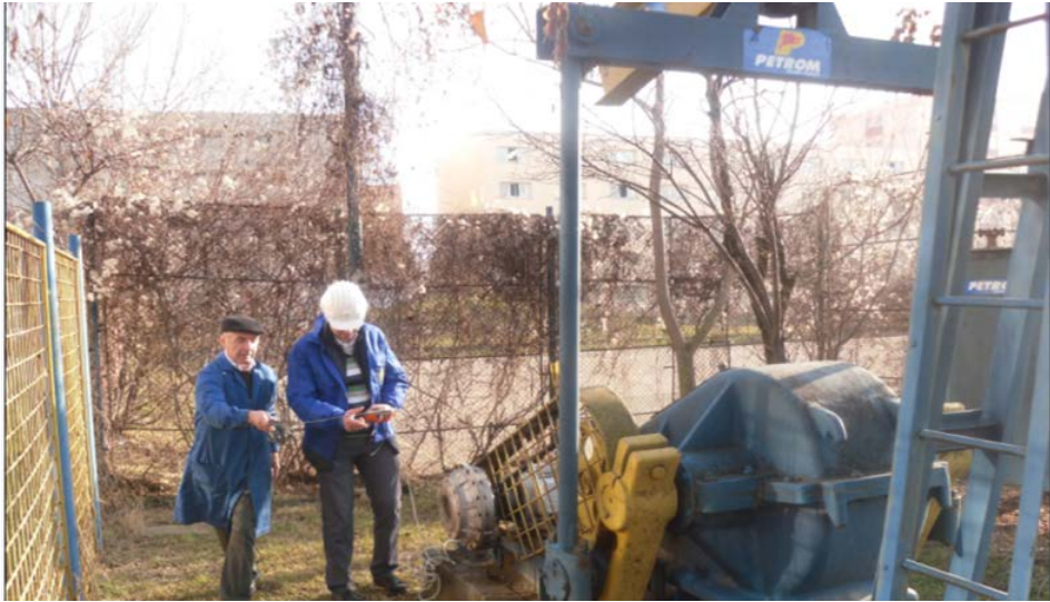
Figure 2. Vibration analysis at the pump unit technical pilot using VIBROTEST 60
