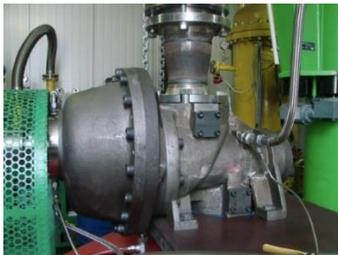
a. CU128GM compressor unit on the INCDT COMOTI test bench
