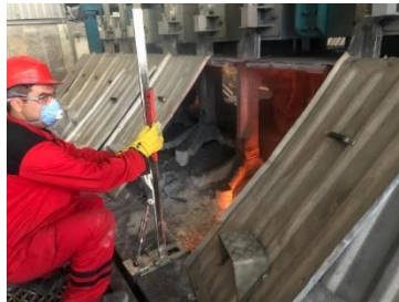
Figure 3. Ledge measurement in an AP12 LE.
