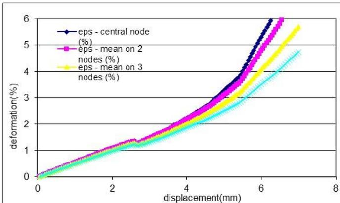
**Figure 6.** Piston displacement - deformation dependency at 400°C, when the fixing holes are drilled on the diameter axis of the big diameter (D) SEU-43 sample
