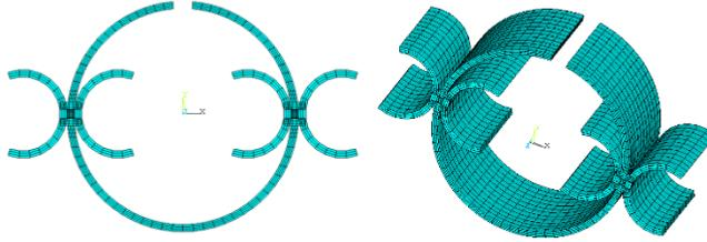
**Figure 1.** Modelling of “C-ring” samples using ANSYS
