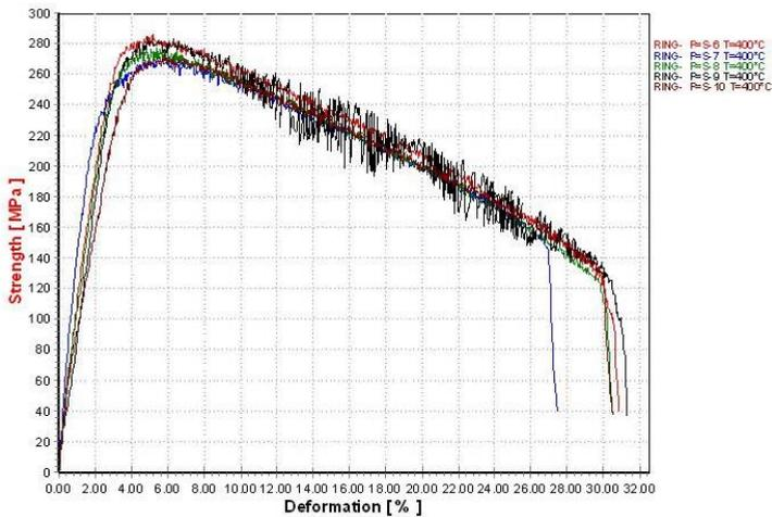
**Figure 5.** The experimental tensile curves for SEU-43 samples, small diameter (d), at 400°C
