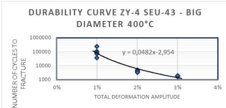
**Figure 8.** Durability Curve for Zircaloy-4, SEU-43, big diameter (D) samples, at 400°C
