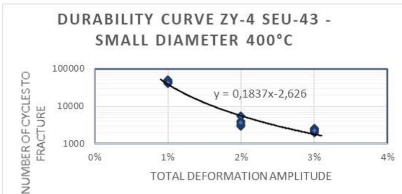
**Figure 9.** Durability Curve for Zircaloy-4, SEU-43, small diameter (d) samples, at 400°C
