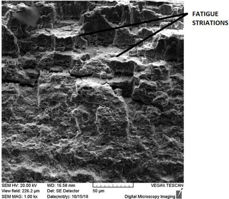
**Figure 10.** Zircaloy-4 break surface of fatigue sample at 400°C (x1000)
