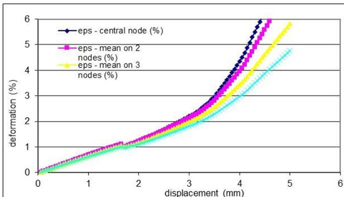
**Figure 7.** Piston displacement - deformation dependency at 400°C, when the fixing holes are drilled on the diameter axis of the small diameter (d) SEU-43 sample
