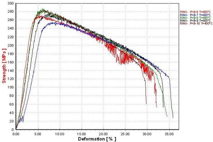
**Figure 4.** The experimental tensile curves for SEU-43 samples, big diameter (D), at 400°C
