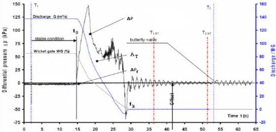
Figure 2. Pressure-time diagram according to IEC 62006
