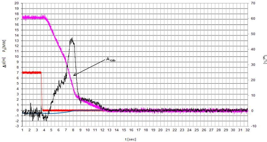
**Figure 5.** Static and dynamic characteristics obtained with Gibson method at a power of 7 [MW]
