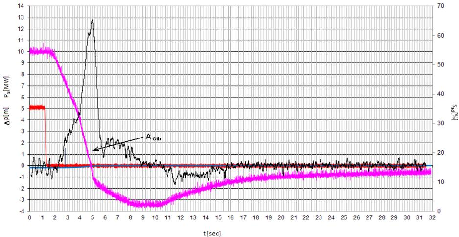
**Figure 4.** Static and dynamic characteristics obtained with Gibson method at a power of 5 [MW]
