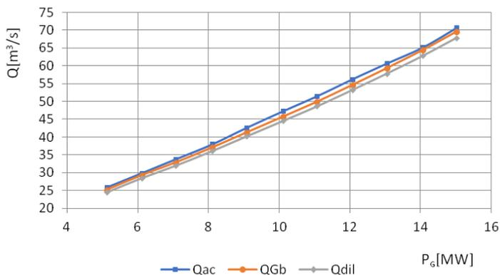
Figure 6. Graphical representation for intake feature  $Q = f(P_G)$  for the 16 MW hydro unit
