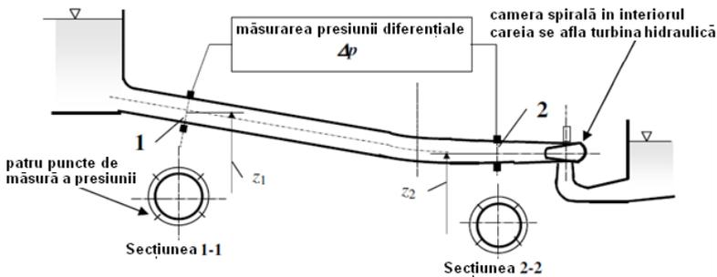
**Figure 1.** Penstock segment with marking of measurement sections required to explain the theoretical basis of the Gibson method [8]
