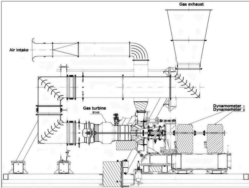
**Figure 4.** Section through the installation of ST40M gas turbine on test bench
