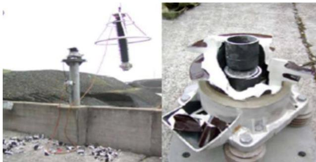
**Figure 5.** Cracking of the metal oxide surge arrester case [8]
