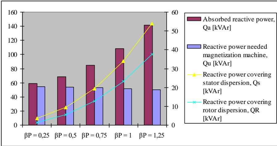
**Figure 4.** Electrical balance diagram of reactive powers in absolute values [kVAr] of studied drive induction motor
