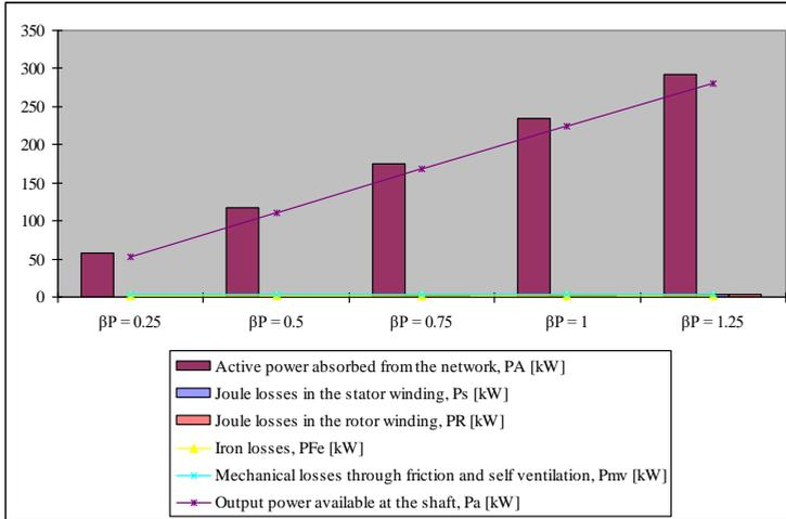
Figure 2. Electrical balance diagram of active powers in absolute values [kW] of studied drive induction motor
