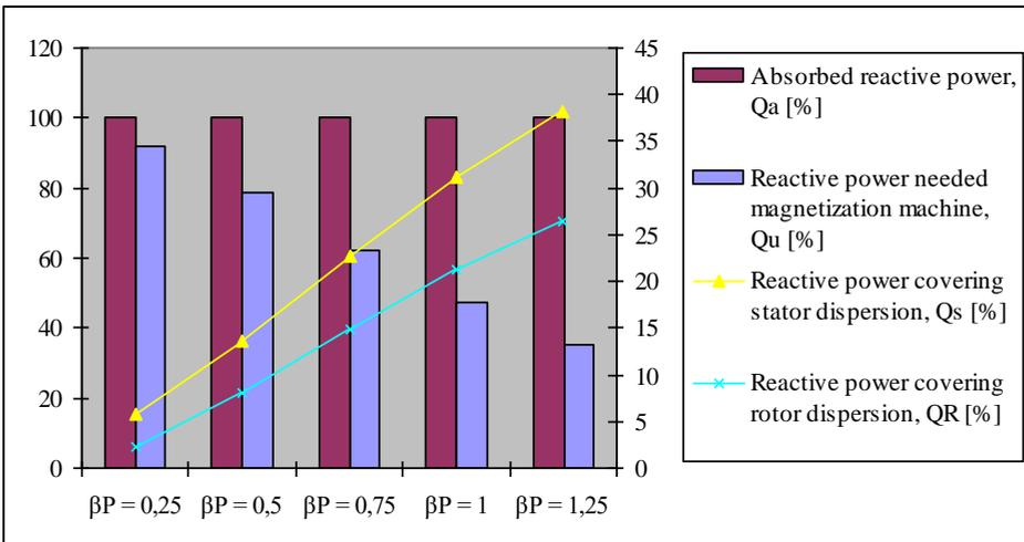
**Figure 5.** Electrical balance diagram of reactive powers in percentage values [%] of studied drive induction motor
