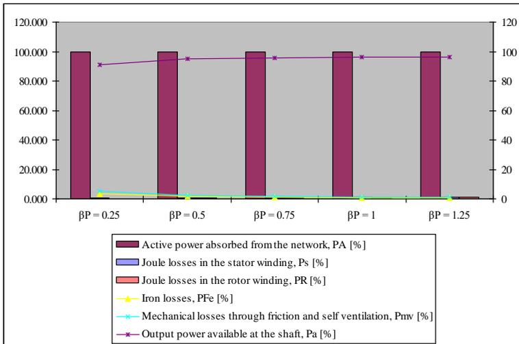
Figure 3. Electrical balance diagram of active powers in percentage values [%] of studied drive induction motor
