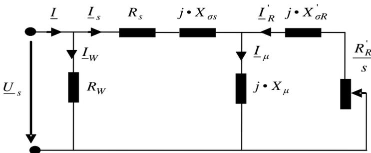
Figure 1. The calculation equivalent scheme for the induction motor.
