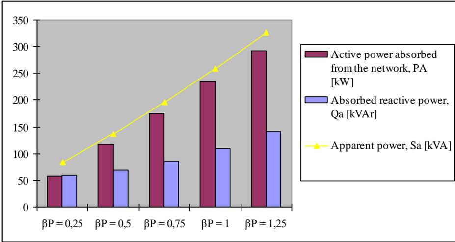
Figure 6. Electrical balance diagram of powers in absolute values of studied drive induction motor
