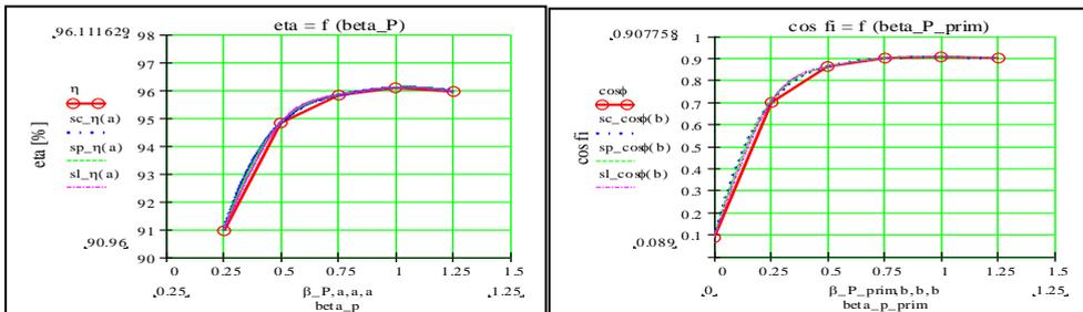
Figure 7. The variation of the energy indicators of the studied drive induction motor according to the load degree
