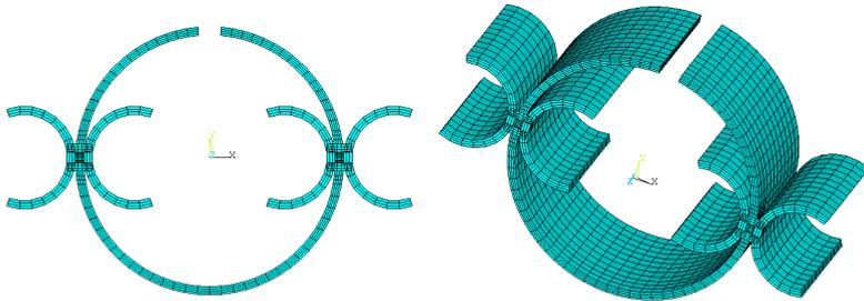
Figure 4. Modelling of “C-ring” samples using ANSYS
